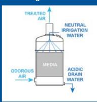
"A vapor-phase odor control technology that uses air-permeable inert media exclusively for the growth of attached microorganisms and the direct biodegradation of odor compounds...irrigation of the media is with clean water."
